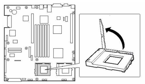
Figure 16 Raising the Locking bar on the socket
